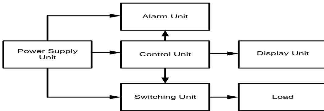
Fig. 1: Block diagram of automatic power selection switch
