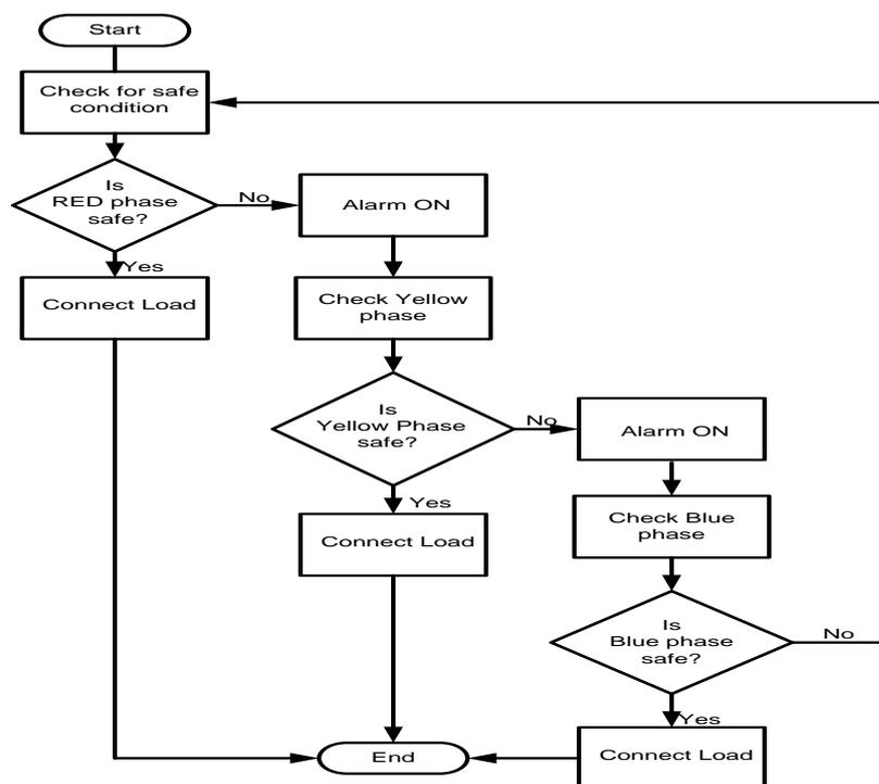
Figure 4: Flowchart of the automatic power selection switch
