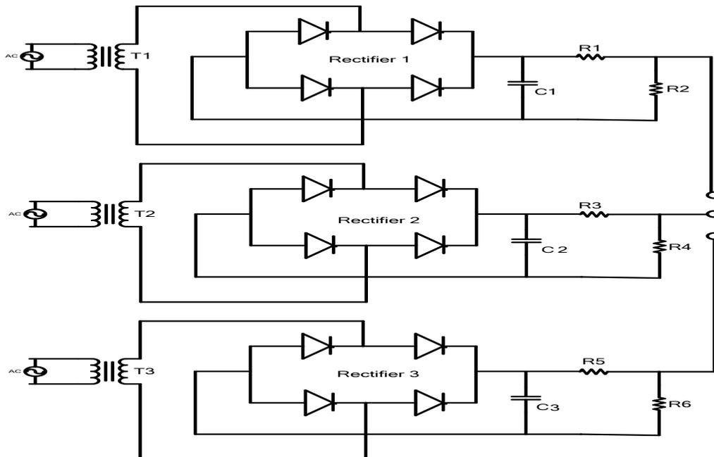
Figure 2: A Three-Phase Power Supply Unit
