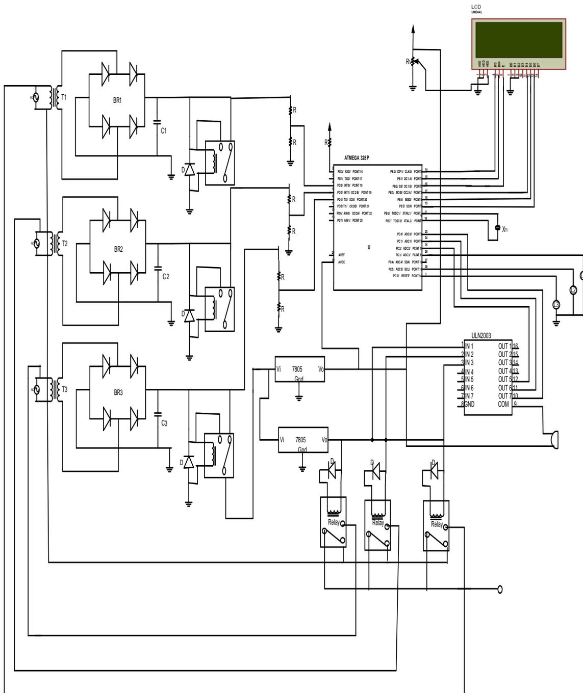
**Figure 3:** Complete circuit diagram for the automatic power selection switch.
